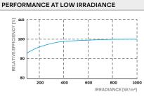
Typical module performance under low irradiance conditions in comparison to STC conditions (25  $^{\circ}C$ , 1000 W/m²).
